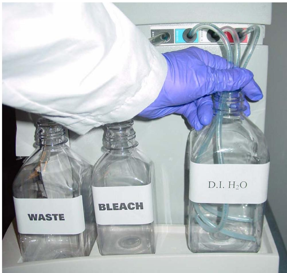
**Figure A.19** Immerse the three wash and water lines in the DI water bottle. The waste line remains in the waste bottle.
