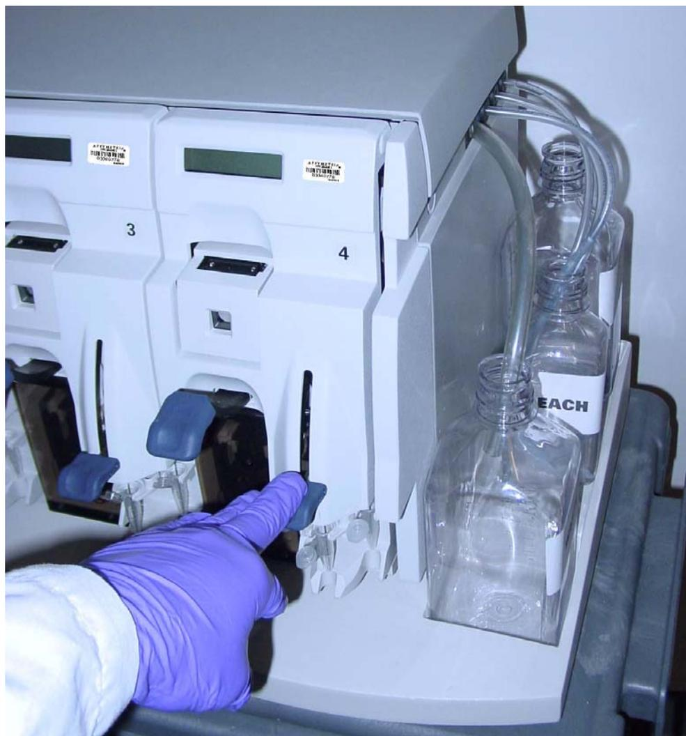
**Figure A.18** Press down on the needle levers to start the bleach protocol.
