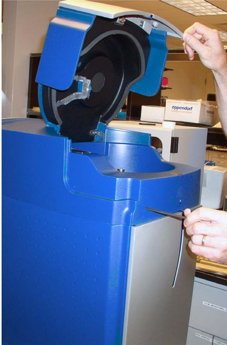
10. Grab and hold the array with your fingers. Using your other hand slowly slide the slot pin (Step 7) back to the left. This should open up the pinch rollers. Pull the array out.
