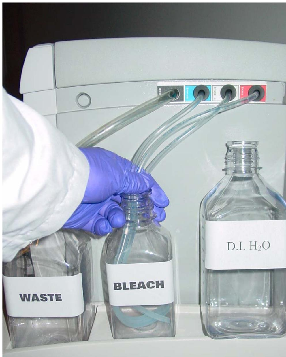
**Figure A.15** Immerse the tubes into the 0.525% sodium hypochlorite solution. The waste line remains in the waste bottle.
