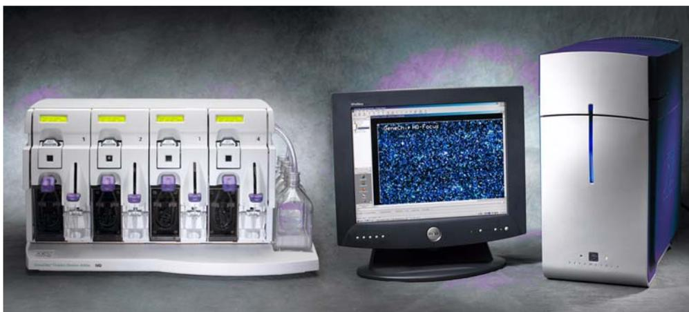
**Figure 1.2** The Microarray Instrumentation System major hardware components: Fluidics Station 450Dx, workstation terminal and GCS3000 Scanner with AutoLoaderDx
