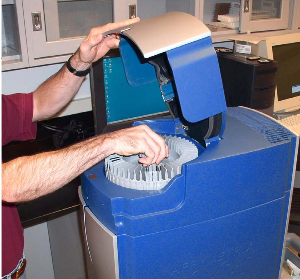
**Figure B.10** Inserting and turning the carousel; the carousel should be seated and flush with housing.
