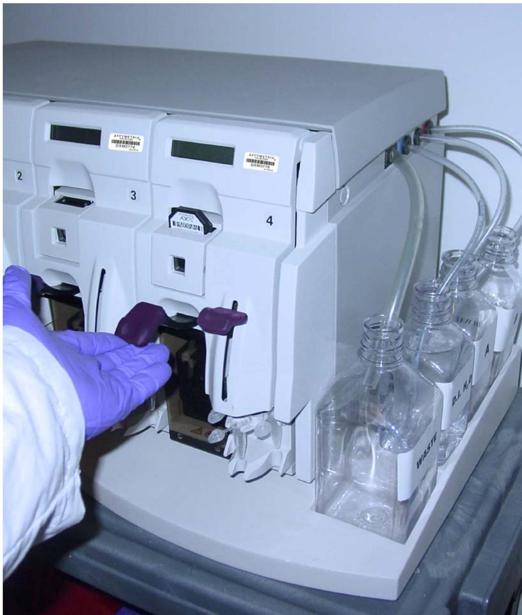
**Figure A.6** Flip the cartridge lever up to engage the cartridge septa needles into the septa.
