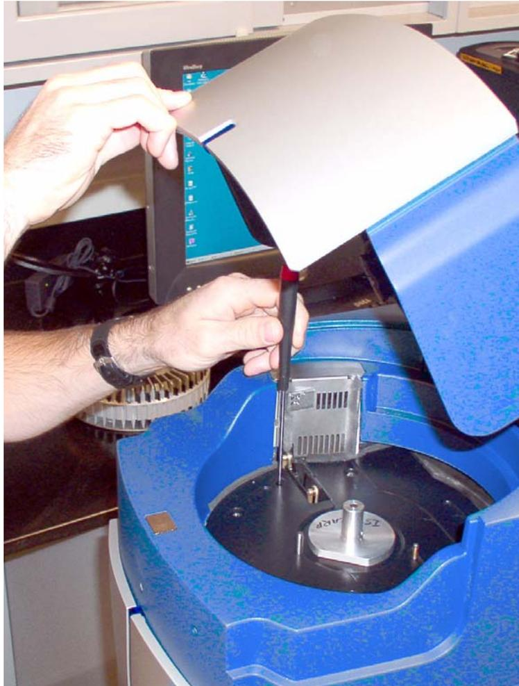
5. Using a standard, flat (-) screwdriver, (13-0257) gently slide it down through the hole making sure not to damage the shaft and spring that are protruding into the hole. When the screwdriver stops, it should be in contact with the scanner Y stage screw. Slowly turn the screwdriver until you feel it engaging the slot on the screw of the scanner Y stage.
