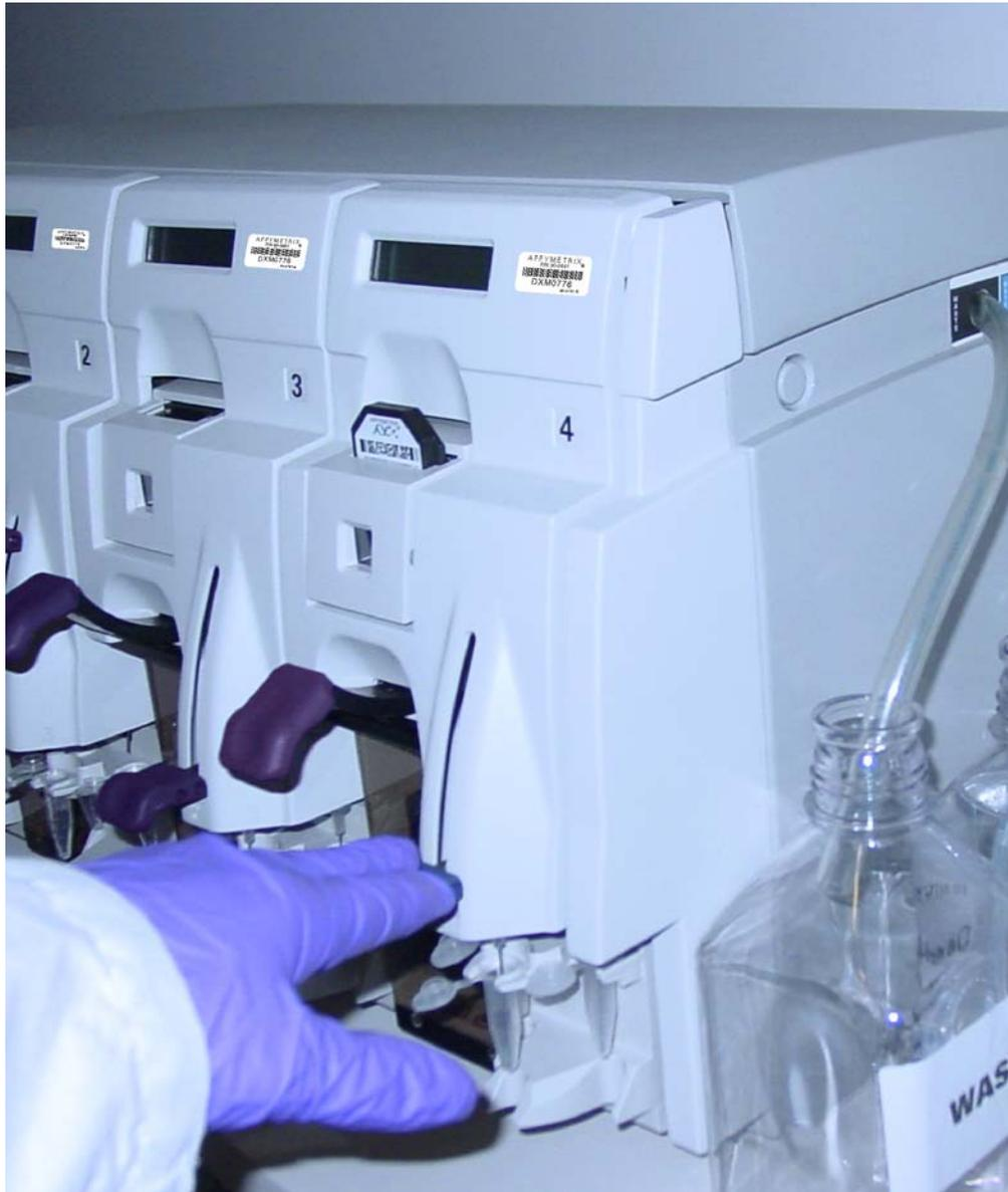
**Figure A.8** Press down on the needle levers to start the protocol.
