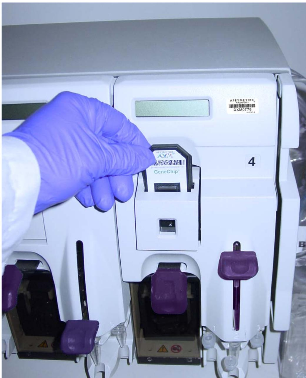
**Figure A.5** Inserting the cartridge into the cartridge holder - note orientation and array label
